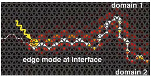
A patterned 'phononic crystal' structure, with snowflake-shaped holes arranged in a lattice, can lead to topological transport of vibrations along edge mode channels. These channels arise at the interface between domains of different geometry.
