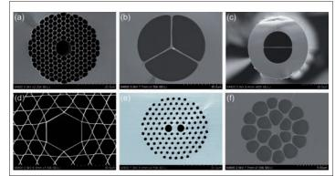
version of the desired structure. This is then drawn down to PCF in two stages, the cross-sectional structure being preserved even after a 1,000 times reduction in scale. The figure shows electron micrographs of a selection of structures produced at MPL (core widths in brackets): (a) hollow core  $(10 \,\mu\text{m})$ ; (b) "Mercedes"  $(2 \mu m)$ ; (c) nanoweb (~500 nm); (d) kagome (28 µm); (e) birefringent  $(3 \mu m)$ ; (f) lead silicate PCF (1.5  $\mu m$ ).
