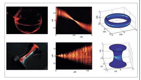
ture – the so-called Gaussian curvature, whereas the topology of the surface has no local effect. We manufactured different bodies with surfaces of constant positive or negative Gaussian curvature. We could demonstrate that a positive Gaussian curvature, as is present on the effects. We thus further develop classical optics while benefiting from the knowledge of general relativity.
