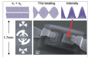
desired THz-frequency and superposed. The resulting modulated intensity is absorbed in a n-i-pn-i-p-superlattice device where it creates the THz-current,  $I_{THz}$ . This current is fed into an antenna which radiates ideally with a conversion efficiency that increases with the laser power squared. To push the roll-off frequencies as high as possible, ballistic electron transport in small area devices is utilized. The advantage of
