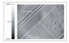
map of a wafer section to illustrate the sensitivity of the method. Microdeflectometry provides appealing pictures, with high lateral resolution, nanometer sensitivity for local surface features, low noise and quantitative 3D features. By combining microdeflectometry with the expansion of the depth of field, we obtain SEM-like images (including quantitative 3D data). The technology is simple, incoherent, and has the potential to rival interferometry.
