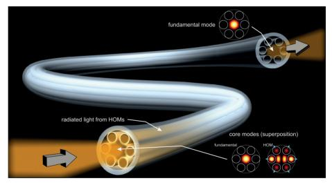
solid-core PCF. We therefore denote this new type of PCF "hESM" (hollow-core endlessly single-mode). Fabricated hESM-PCFs show 15× higher HOM suppression compared to kagomé-style PCFs. They are very useful for applications in which  $M^2 \sim 1$  beams are
