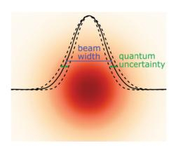
remarkable because it shows that the uncertainty in a geometrical characteristic depends on the quantum properties of the light. Moreover, we have discovered the interesting fact that the uncertainty in beam-width stems entirely from noise in the amplitude quadrature of one specific mode that is uniquely given by the field under investigation. Reducing the uncertainty in amplitude quadrature of this mode reduces the beam-width noise.
