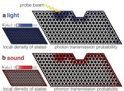
chiral sound waves. The light can be used at will to change the topological properties and redirect the sound waves on the chip. These ideas may be implemented in optomechanical crystal devices and contribute to fundamental studies of phonon transport.
