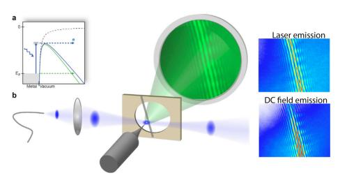
periment was realized, see image. The resulting interference pattern was detected, in one case for DC field emission, in the other for photo-emitted electrons. Both images show clear interference fringes, directly indicating the electron coherence. Hence photo-emitted electrons are (al-
