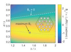
which the circular birefringence is maximum (see figure). This result was then confirmed experimentally by drawing PCFs with a range of different geometries. The current measurements showed excellent linearity over the working range in agreement with theory. Twisted PCF is therefore ideal for building magnetic field and current sensors based on the Faraday effect.
