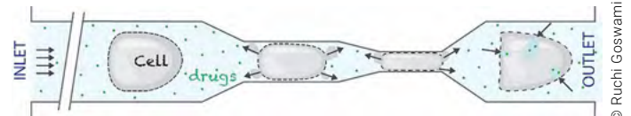
The cells are stretched by passing through the nanochip. This creates pores in their cell membrane, allowing molecules to pass through and get inside the cells
