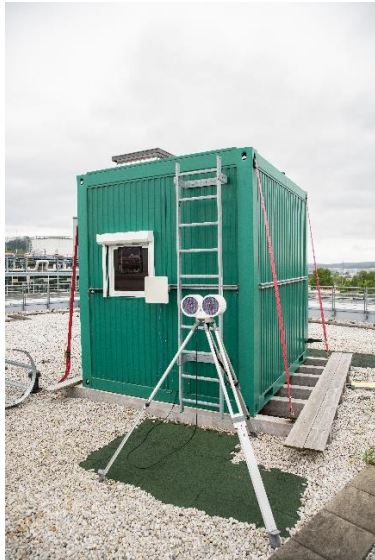
A green container on the roof of the Jena municipal utility houses the telescope for sending the quantum keys. The Fraunhofer IOF is located 1.7 kilometers away as the crow flies. © Fraunhofer IOF
