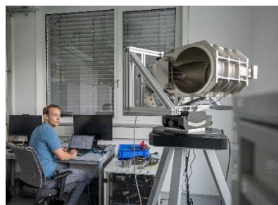
A special metal mirror telescope is used to distribute quantum keys via free-space. © Fraunhofer IOF
